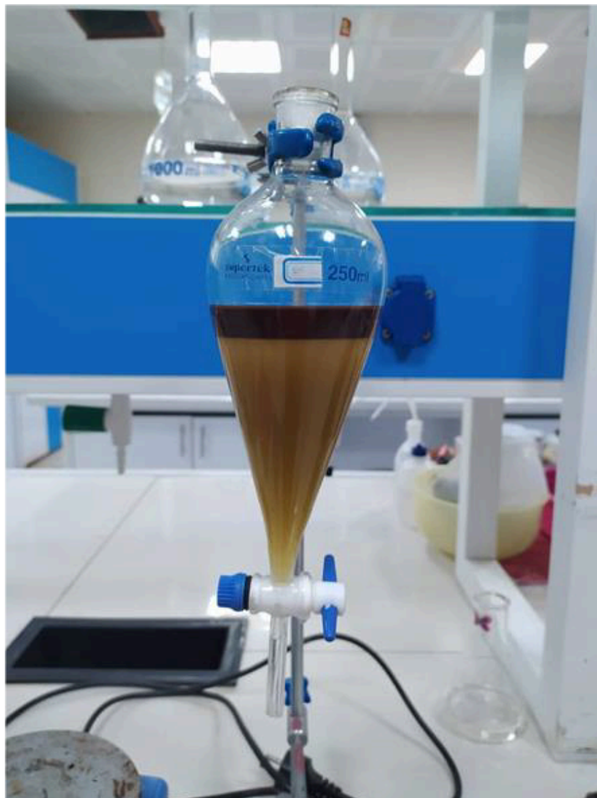
Fig. 1. The two-phase system of biodiesel and un-reacted methanol.
